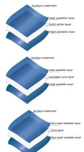
**FXCP** is coextruded pearlized BOPP film with very high gloss, both sides heat sealable, one side corona treated with very high yield and low density. Reduces the costs for packing.
