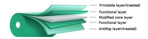
The Anti-fog properties are sensible of the storage time and conditions, that's why is advisable FXCAF to be used not later from 6 months after delivery date. The Anti-fog layer is not suitable for printing.
